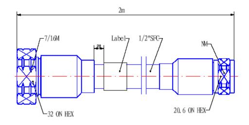
d. Cable : 1/2" super flexible cable Bending radio : 40mm
